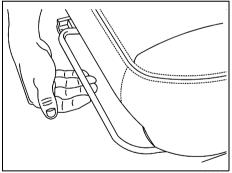
Lift the bar located under the front of the seat to unlock it. Slide the seat to where vou want it and release the bar. Try to move the seat with your body to be sure the seat is locked in place.
